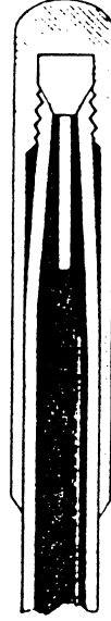
No. 8. Sectional view of cap, showing cone in the tip which plugs end of nozzle, making it air tight.
